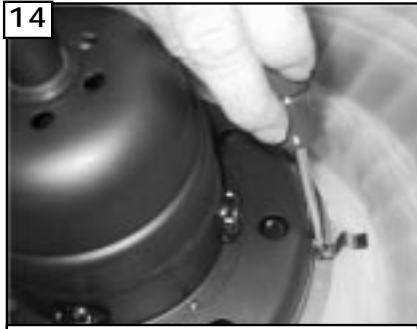
Install 3 screws and clips to hold glass to fan housing.
